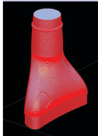
Figure 1 - FDM sacrificial tooling is easily created from the CAD model of the composite part and prepared for building using Stratasys Insight software.
