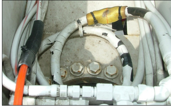
Turtable bearing bolts in place and torqued, Pedestal to bearing and turtable to bearing
