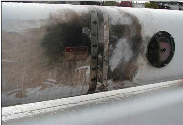
Electrical contact – Arc marks –
