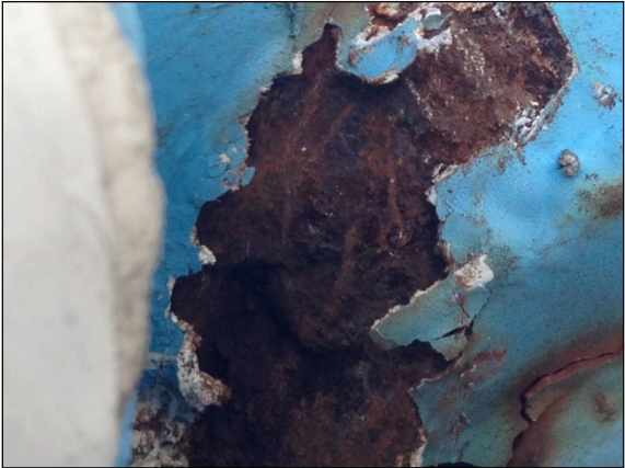
Severe rust hiding a crack. Inspection requires cleaning the area
