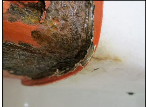
Severe rust and fiberglass crack
