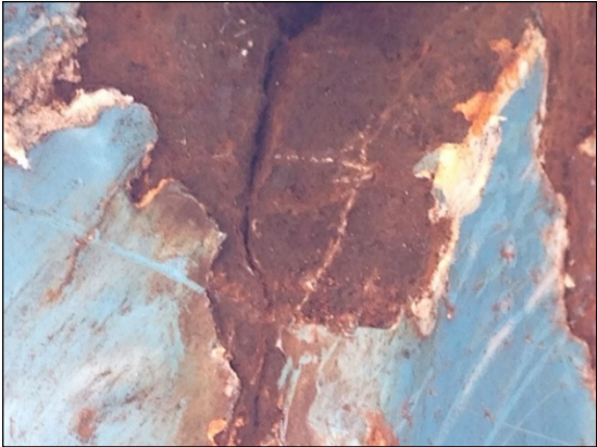
Severe rust hiding a crack. Inspection requires cleaning the area
