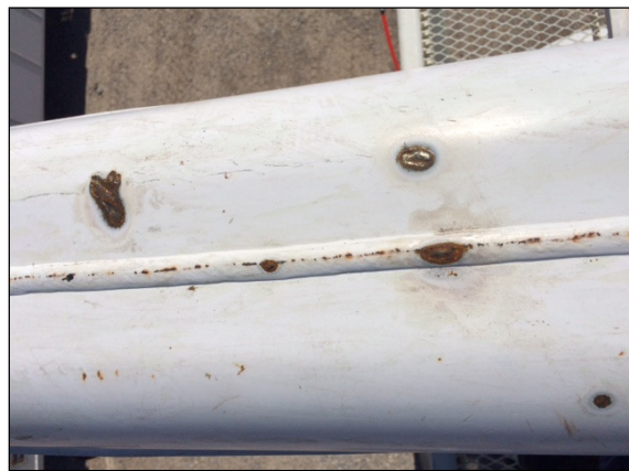
Electrical contact – Arc marks –
