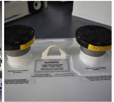
2 Emergency vents opening
