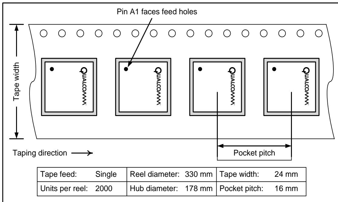
**Figure 5-1 Carrier tape drawing with part orientation**
