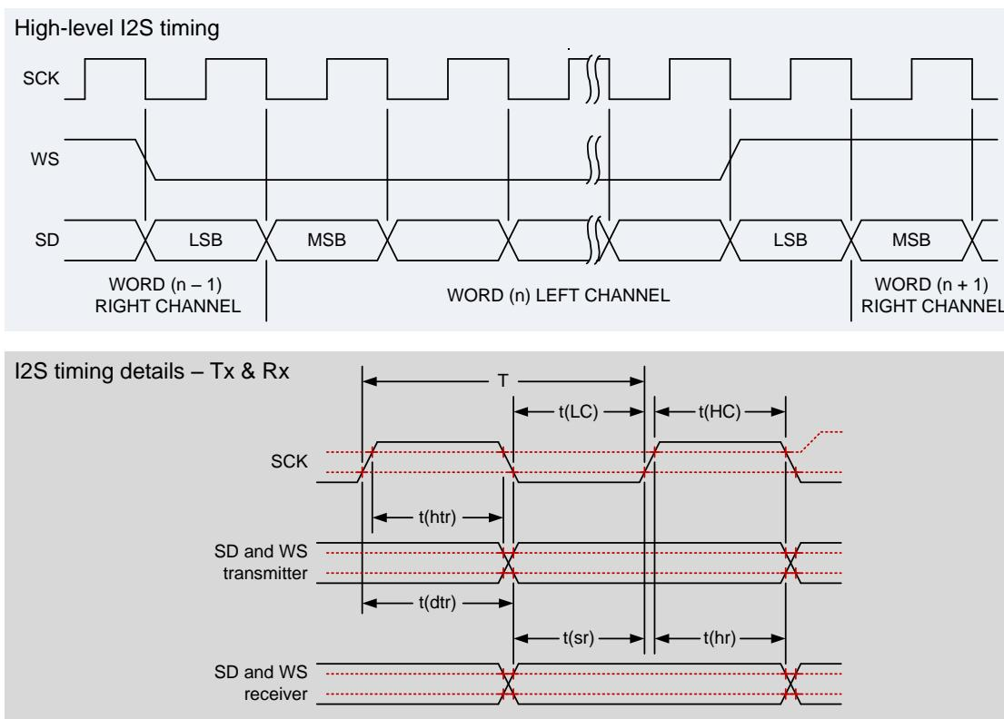
Figure 3-13 I<sup>2</sup>S timing diagramTable 3-26 I<sup>2</sup>S interface timing
