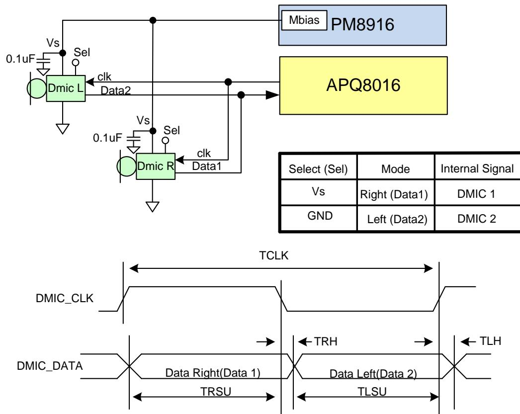
Figure 3-14 APQ8016E digital mic PDM interface timing
