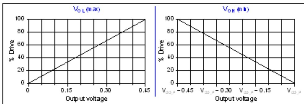
**Figure 3-1 IV curve for V<sub>OL</sub> and V<sub>OH</sub> (valid for all V<sub>DD\_Px</sub>)**
