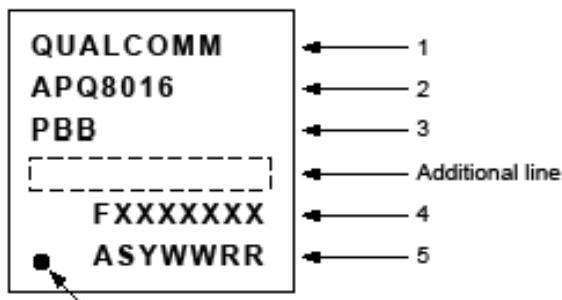
Figure 4-2 APQ8016E device marking (top view, not to scale)
