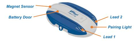
**Remote Control:** The Remote Control (model PTRC3000T) is a handheld, battery-operated unit that communicates with the Trial Stimulator using Bluetooth<sup>®</sup> wireless technology. The patient can use the Remote Control to turn stimulation on or off and adjust certain therapy settings, as well as retrieve the current stimulation level and battery status from the Trial Stimulator.
