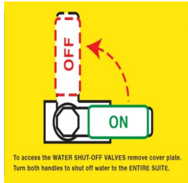
This sticker will help you locate the main water shut off valve in your suite.
