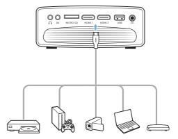
2 Press → to display the input source list, and then select HDMI 1 or HDMI 2.
