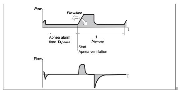
Apnea ventilation corresponds to the SIMV ventilation mode with AutoFlow.
