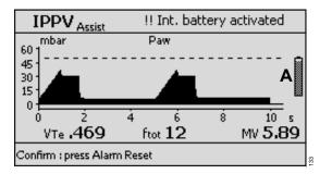
Wait about 30 seconds. The remaining capacity display (A) indicates the charge state of the internal battery.
