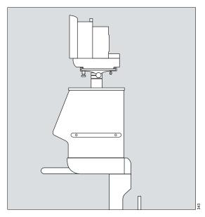
Mount the Infinity monitor onto Savina using the corresponding holder.
