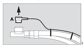
2 Remove the breathing gas temperature sensor (A) from the Y-piece or from the holder of the breathing circuit for pediatric patients. Do not pull on the cable.
