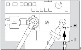
Connect the nebulizer hose (I) onto the nebulizer port (H).
