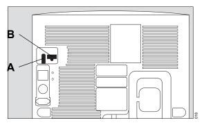
3 Remove the fuse (B) for the internal battery and place it in the storage recess (A).
