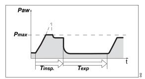
If pressure limitation *Pmax* is enabled, pressure peaks are avoided. Ventilation mode PLV is thus realized.
