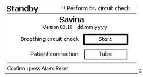
On the Breathing circuit check line select the Start setting with the rotary knob and push to confirm.
