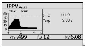
While setting a ventilation parameter, derived ventilation parameters are calculated and displayed in the setting assistance field of the main screen.
