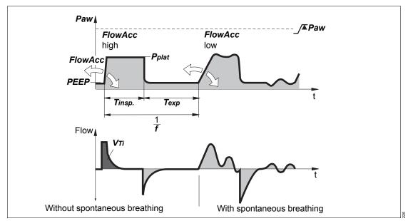
Savina provides ventilation with AutoFlow with a decelerating flow in order to avoid pressure peaks. Savina determines the pressure required for the set tidal volume, taking into account the condition in the lungs (compliance, resistance) and the patient's spontaneous breathing demand.
