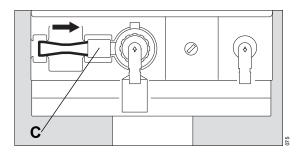
3 Push the flow sensor as far to the right as it will go into the flow sensor sleeve (C) of the expiratory valve.
