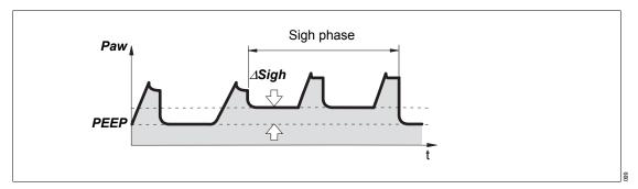
Atelectasis can be prevented by activating the sigh function and setting the sigh in the form of an intermittent PEEP. The purpose of expiratory sigh is to open collapsed areas of the lungs or to keep open slow areas of the lungs.
