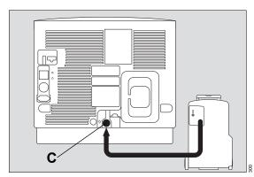
Connect the O2 supply hose of the oxygen source, e.g., O2 concentrator, to the LPO inlet for low pressure (C).
