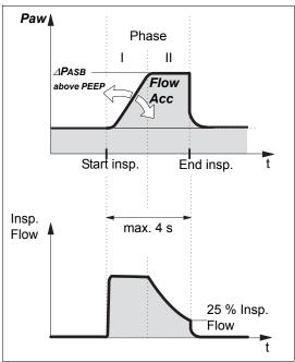
Pressure support is initiated when the flow trigger is triggered.
