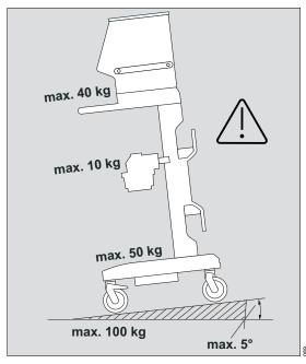
The maximal total load of the trolley must not exceed 100 kg (220 lbs).
