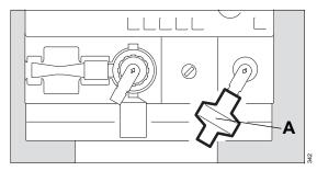
Fit the bacterial filter (A) onto the inspiratory port.
