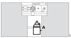
Hang the breathing gas humidifier on the humidifier holder (A) using the clamp and screw firmly into place.
