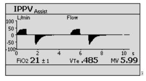
For *FiO*<sub>2</sub>, both the measured value and a tolerance (±) are displayed. See page 201 for a detailed description.
