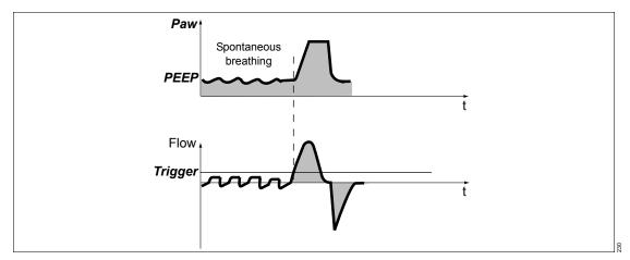
With the trigger threshold *Trigger*, the mandatory breaths and pressure support  $\triangle PASB \ above \ PEEP$  are synchronized with the inspiratory efforts.
