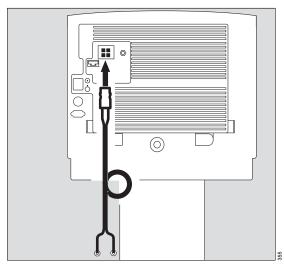
Connect the external battery with the battery cable (8414092) or connect the DC on-board power supply with the on-board power cable (8414048).
