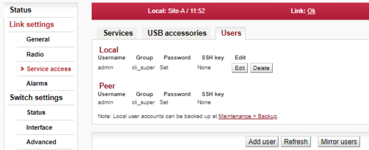
Fig. 3.5: Configuration menu Link settings / Service access / Users
