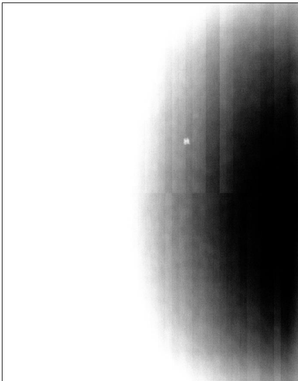
Artefacts created by the presence of object on filter, mylar mirror or Be window.
