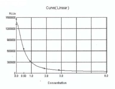
Free T4 concentrations are calculated by using a calibration curve. This method utilizes a four parameter logistic curve with an inverse relationship of measured light produced (RLU) to concentration of free T4 in the serum sample. Serum results are expressed as mg/dL.
