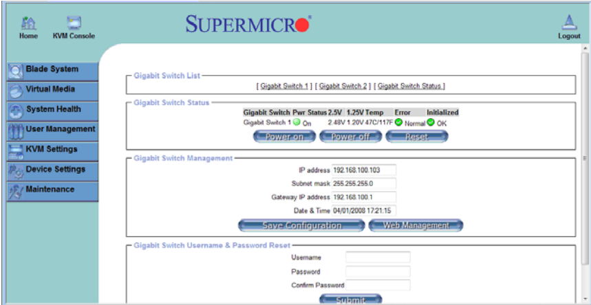
Figure 6-1. Switch Status Screen
