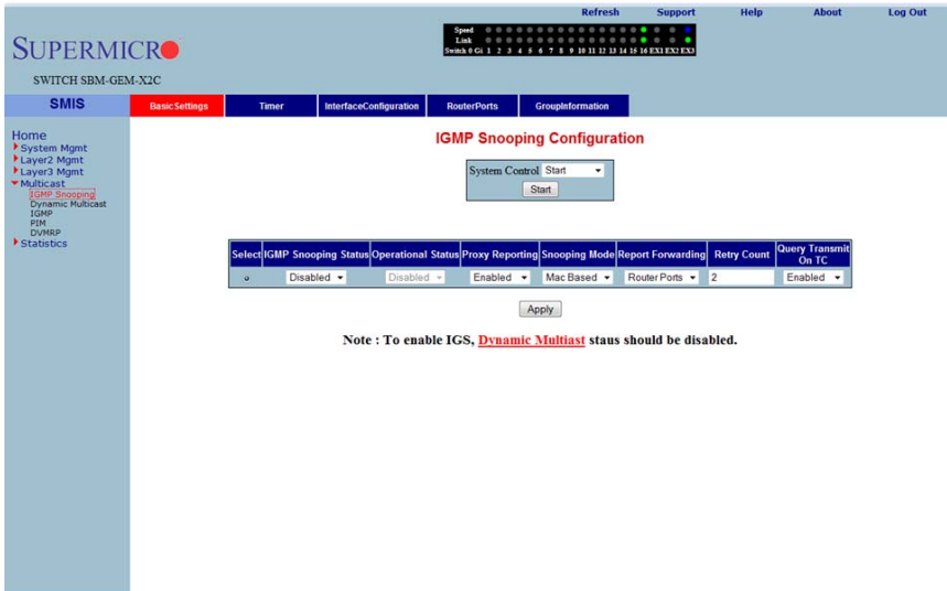
Figure 7-148. IGMP Snooping Configuration Page
