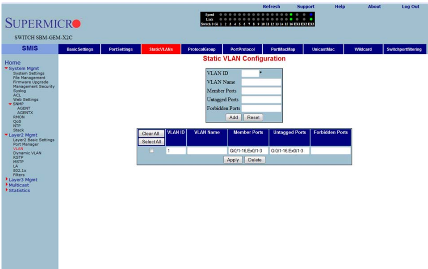
Figure 7-63. Static VLAN Configuration Page
