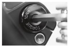
1. Slide in the axle and tighten it with a 6mm Allen wrench by suggested tightening torque of 10Nm.
