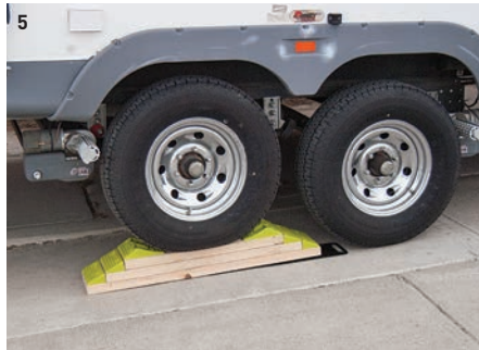
4, 5) To lift the trailer, the stacked boards are placed in front of or behind the wheel(s) and the trailer is pulled or backed until the wheel(s) are secure between the docks on the top board. Two kits are needed to lift both wheels on a tandem-axle trailer (not shown).
