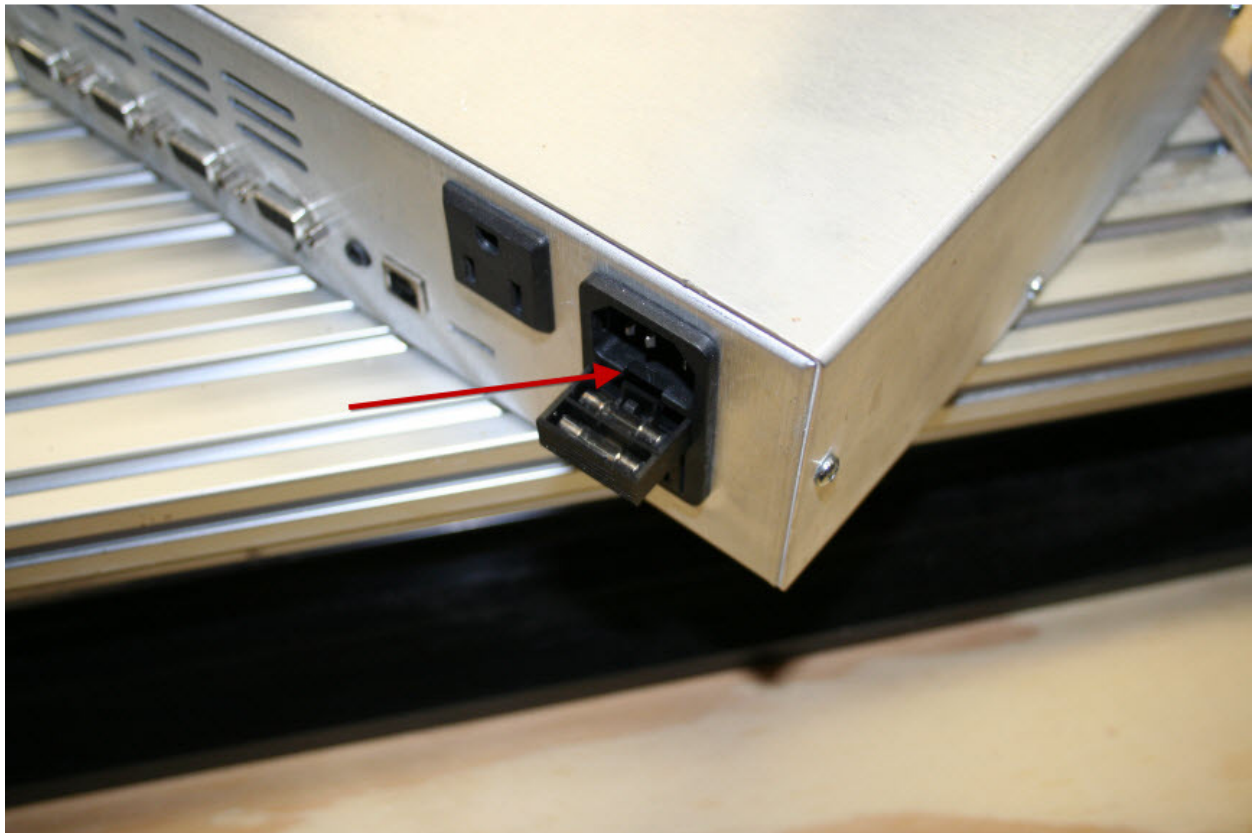
Figure 158 - Shark Control Box Power Cord Fuse
