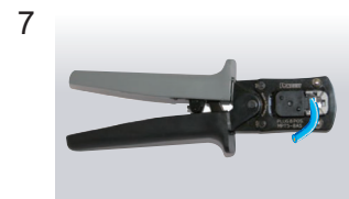
7 Using special crimping tool MPT5-8AS (PANDUIT CORP.), crimp the modular plug. Finally check the plug visually.
