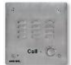
W-3000 Faceplate: Vandal resistant 14 gauge louvered 316 marine grade stainless steel with #4 brushed finish and laser etched graphics. Optional VE-5X5 surface mount box available (page 33).
