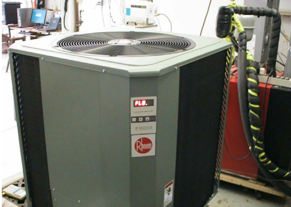
Figure 23 Rheem Model 8320ti electric heat pump being tested at BNL
