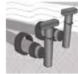
Fig. 8.4 Low point drains
