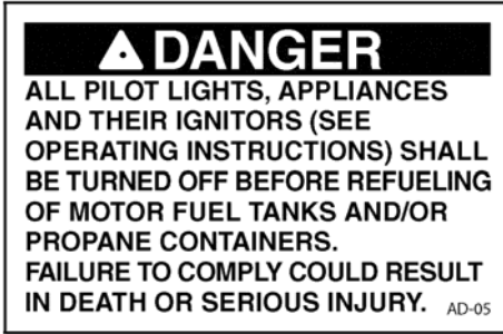
Fig. 7.9 Refueling warning label
