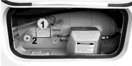
1: Propane fill valve; 2: Propane gauge Fig. 7.4 ASME tank
