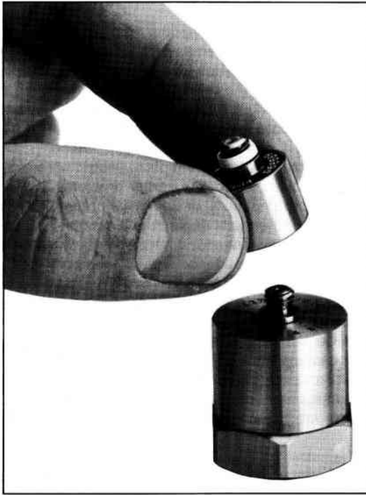
Fig. 3.17. Attaching the Line-drive Amplifier Type 2644 to the top of an accelerometer
