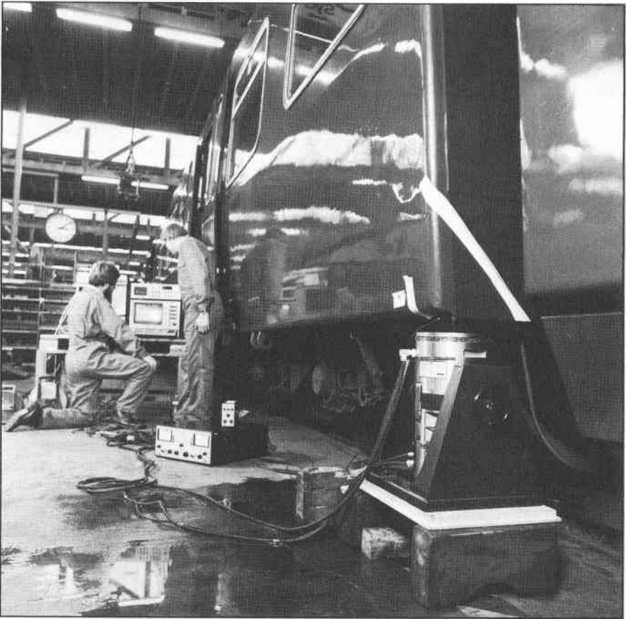
Fig. 1.3. The structural analysis of a train carriage using vibration measurements
