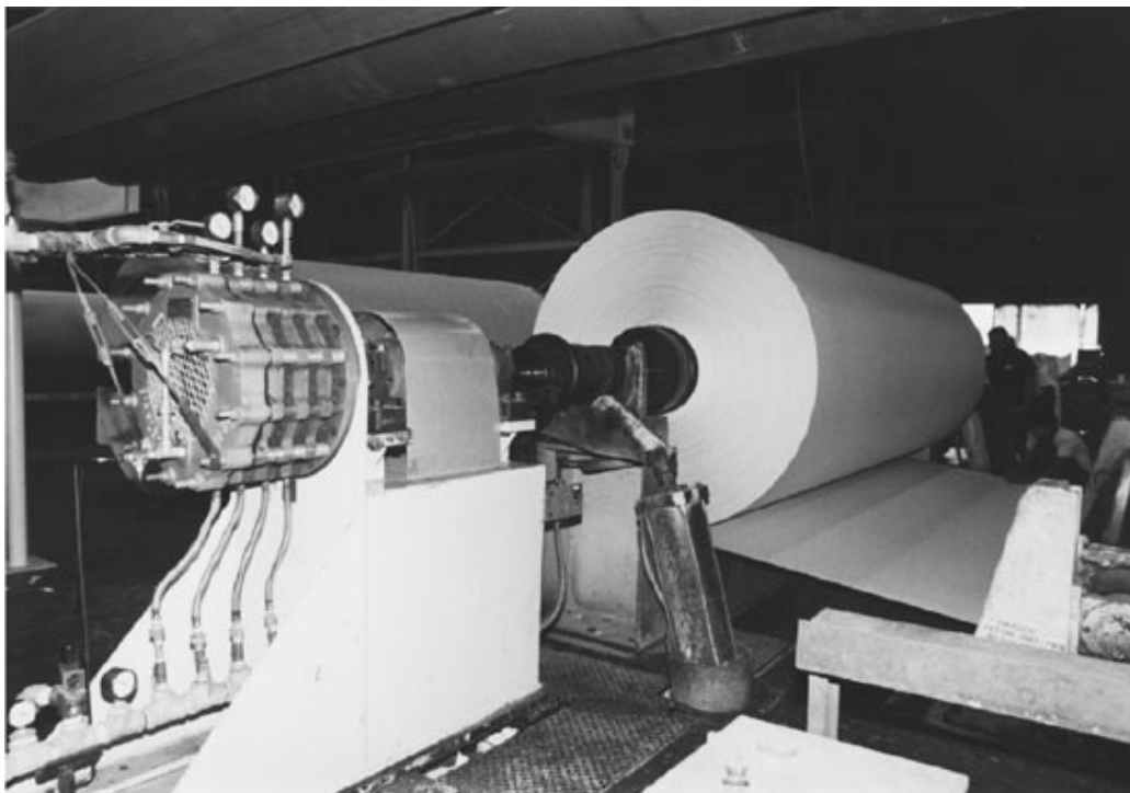
318WCB tension brake on paper unwind stand 65 lb paper (30 kg), 178 inch (4,5 m) @ 5500 fpm (25,4 mps).
