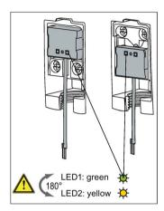
Figure 4-2 LED element rotated 180°
