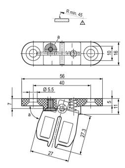
Figure 4-7 3SX3256 radius actuator, radius adjustable
