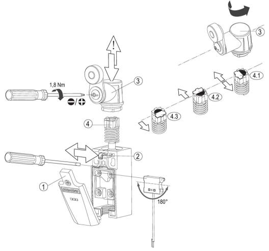
Figure 4-3 Changing the actuator head (example: part-turn actuator)
