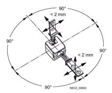
Minimum force requirement in direction of actuation 30 N (when withdrawing)
