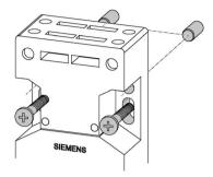
To avoid shifting on approach from above, optional fixing bolts can be used for precise adjustment.
