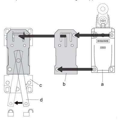
Figure 5-1 Quick-release device
