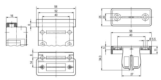
Figure 4-9 3SX3234 separate actuator with dust protection and slit covers
