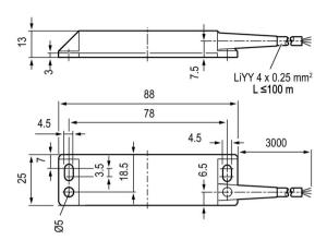
Rectangular contact block, 25 x 88 mm, with M12 plug, 3SE6604-2BA01 / 3SE6605-2BA01
