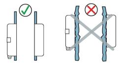
The safety sensor and the actuator must be mounted inseparably on the protective device.
