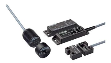
A magnetically operated switch comprises a coded switching magnet and a contact block (sensor unit). Evaluation requires a safety relay or connection to a bus system.
