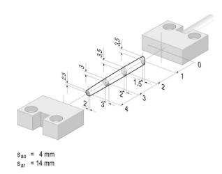
$s_{ao}$  = safe operating distance ON  $s_{ar}$  = safe operating distance OFF
