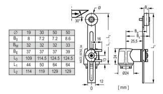
$v_{(met)} \le 1.5 \text{ m/s (maximum actuating speed)}$
