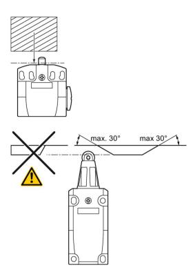
Installation instructions for position switches with roller lever, angular roller lever, twist lever, and rod lever
