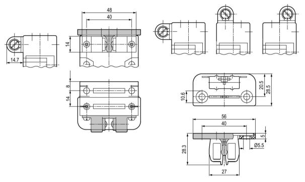
Figure 4-8 3SX3217 separate actuator with ball locating
