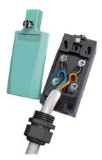
These position switches have an option for easy and fast wiring. The connecting cable is first connected to the contact block terminals and then routed through a slot in the cable gland opening.
