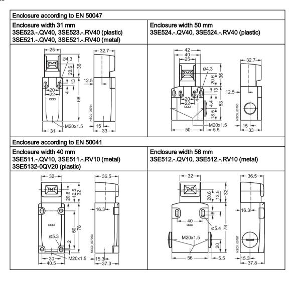
4.5 Mechanical safety switches with separate actuation
