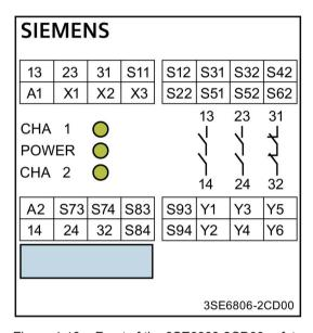
Figure 4-16 Front of the 3SE6806-2CD00 safety relay
