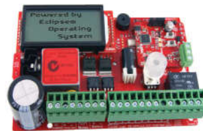
Control card with Eclipse® Operating System
