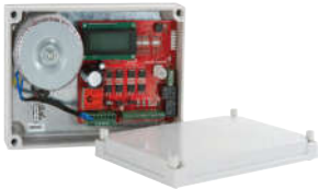
Intelligent control box with built-in receiver
