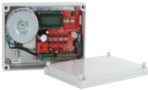
Intelligent control box with built-in receiver.
