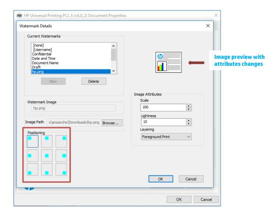
• Scaling: This option allows to scale in or out the watermark by selecting the appropriate value. The valid range is 10-999.
