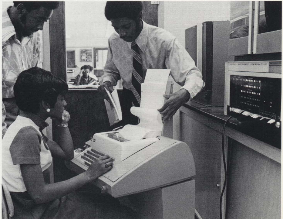
The Digital PDP-8 computer with teletype was one of the earliest computers introduced into public schools.
