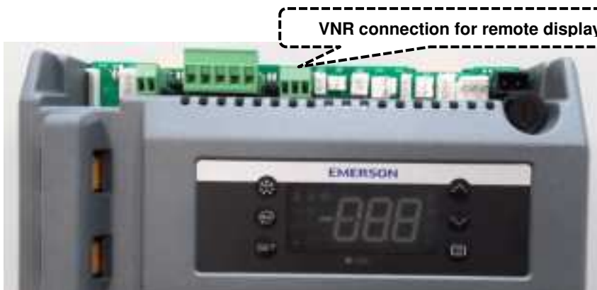
Figure 12: VNR connection for the remote display
