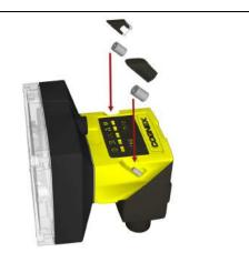
6. After each cap nut has been fastened, torque to 0.12 Nm (1.06 in-lb) and reinstall the screw covers.
