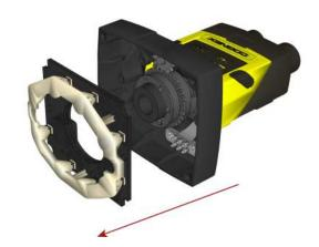
5. Carefully align the connector on the back of the new LED ring light with the pins on the vision sensor. Gently press down the LED ring light to the optics module.
