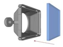
5. Reinstall the filter holder back to the front cover, tightening the screws until they stop turning.
