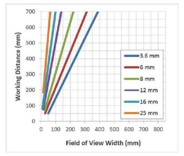
The following chart shows the horizontal field of view for In-Sight 2000-130 vision sensor with 800 x 600 image resolution (2X Image Magnification mode).
