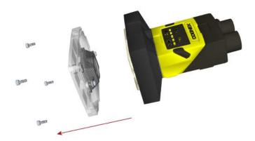
3. Move the lens to the furthest out position by turning the screw on the back of the light module clockwise.
