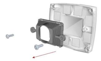
4. Hold the filter by the sides, then push the filter in until it is sitting firmly against the filter holder.
