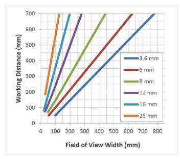
The following chart shows the horizontal field of view for **In-Sight 2000-120/130** model vision sensors with 640 x 480 image resolution in 2X Image Magnification mode.
