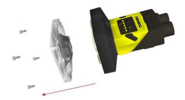
3. Unscrew the two screws on the filter holder and remove the filter holder from the front cover.
