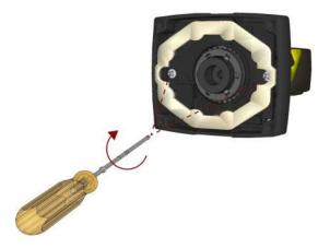
7. Reattach the front cover. Tighten all four screws using a torque wrench; the maximum torque is 0.2 Nm (1.77 in-lb).
