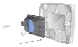
6. Reattach the front cover. Tighten all four screws using a torque wrench; the maximum torque is 0.2 Nm (1.77 in-lb).
