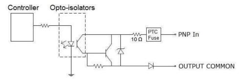
For PNP lines, the external load should be connected between the output and the negative supply voltage (0VDC). When connected to a 24VDC power supply, the outputs pull up greater than 21VDC when ON, and current flows through the load. When the outputs are OFF, no current flows through the load. For more information, refer to <a href="Power and I/O">Power and I/O</a> Breakout Cable Specifications on page 30.
