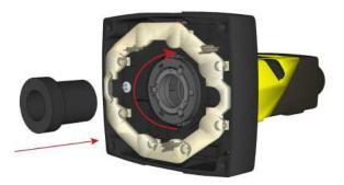
6. Reattach the front cover. Tighten all four screws using a torque wrench; the maximum torque is 0.2 Nm (1.77 in-lb).
