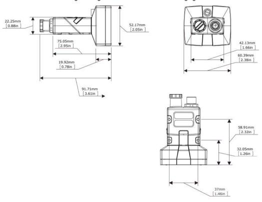
The size of the vision sensor in the angled configuration is shown in the following figure:
