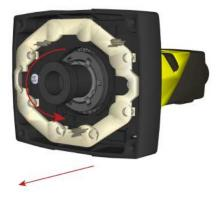
5. Insert the new lens and using your fingers, turn it clockwise to tighten the lens.
