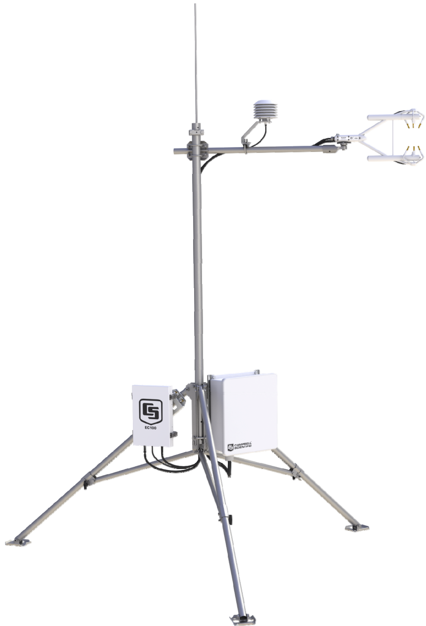
FIGURE 2-1. Open-Path Eddy-Covariance (IRGASON) System
