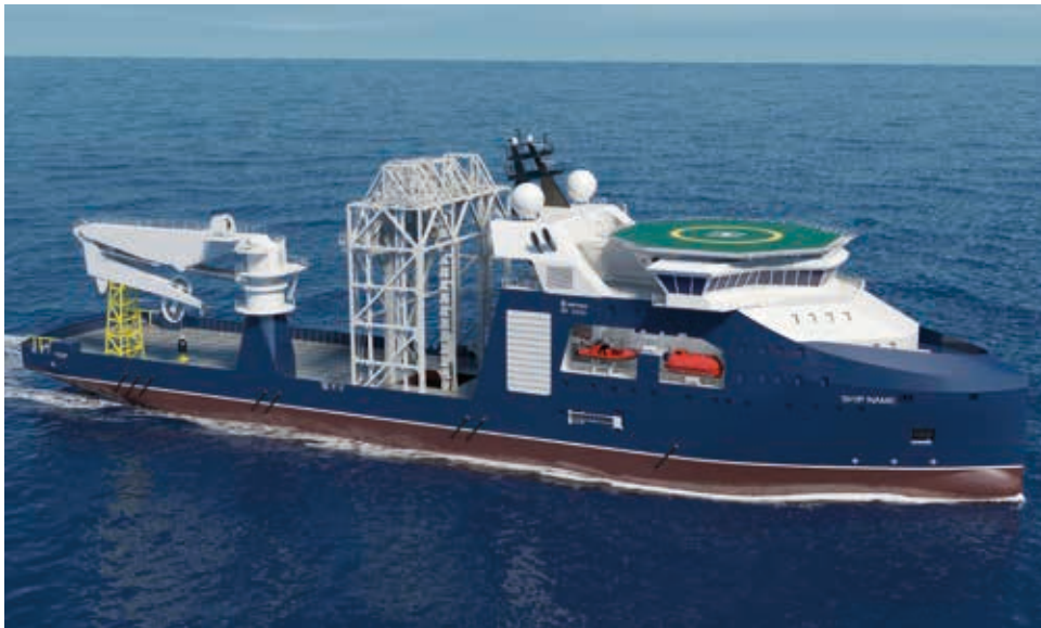
ABOVE: The UT XXXX SCV is a series of different size vessels. The size is mainly determined by the capacity of the offshore crane, which can be from 150 to 600 tonnes.
