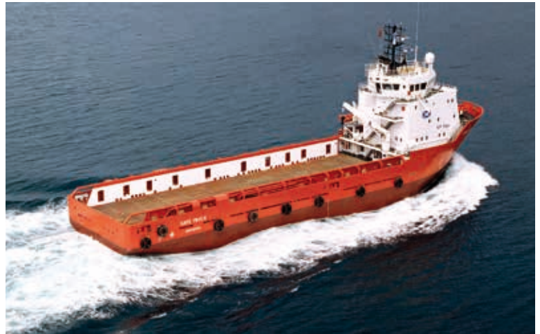
ABOVE: Since its introduction in the 1990s, the UT 755 has grown to be the most popular supply boat yet, with 160 now in service. Long and short versions have been introduced to match market requirements.
