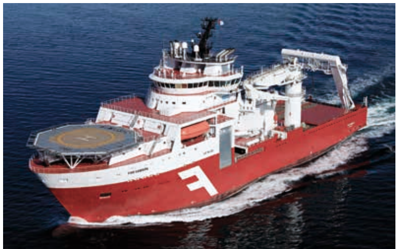
TOP: The UT 712 anchorhandling vessel Olympic Octopus was the world's most innovative when it entered service in 2006, with an array of safer deck equipment, DP2 and automation.
