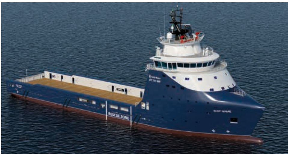
BELOW: The UT 771 WP complements other PSV designs and can carry a range of cargoes in a safe and efficient way. It has a deadweight of 4,200dwt.
