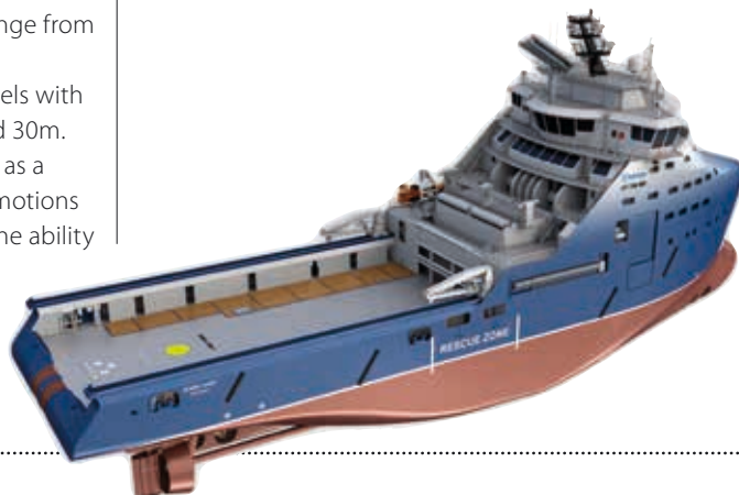
BELOW: The UT 790 WP anchorhandler has a bollard pull of 250 tonnes, scalable to meet customer requirements.
