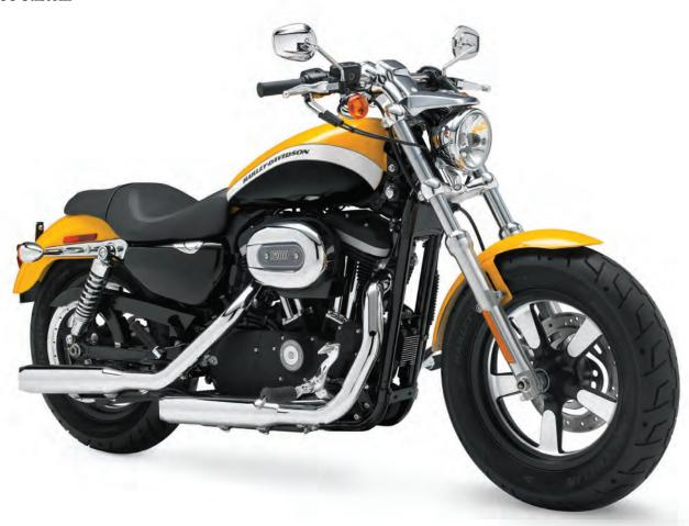
he 1200 Custom comes equipped with Chrome, 5-spoke Cast Aluminum wheels; pull-back handlebar; forward polished foot controls; a two-up seat; black engine with chrome covers; and Vivid Black paint.
