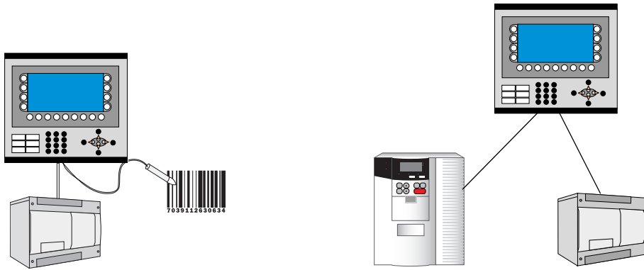
Operator terminal with control system and barcode reader connected.
