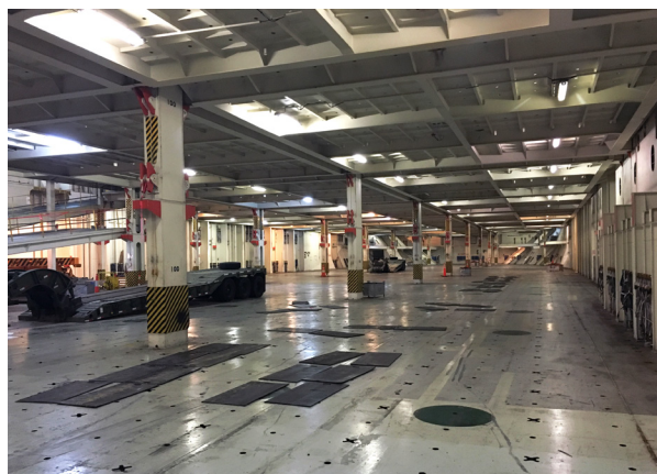
The interior of the MV Green Bay provides 189,000 sq. ft. for transporting high and heavy military cargo and equipment.
