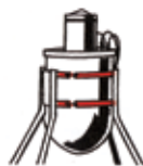
This precision instrument is sealed by a V-Band Coupling and supported by a Band Clamp assembly.
