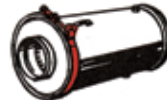
Klystron tube is water cooled; V-Bands keep water jacket tight but easily accessible for maintenance.
