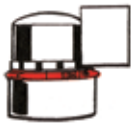
Motors assemble with uniform stresses when housings are joined with V-Band Couplings.
