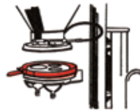
Interchangeable cheese molds clamp quickly onto this machine with Over Center Latch Coupling.
