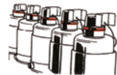
Central vacuum sweepers use motors assembled and sealed by a V-Band Coupling.
