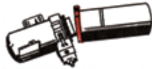
Coupling with one screw assemblies and seals pump, valves, motor and tank.
