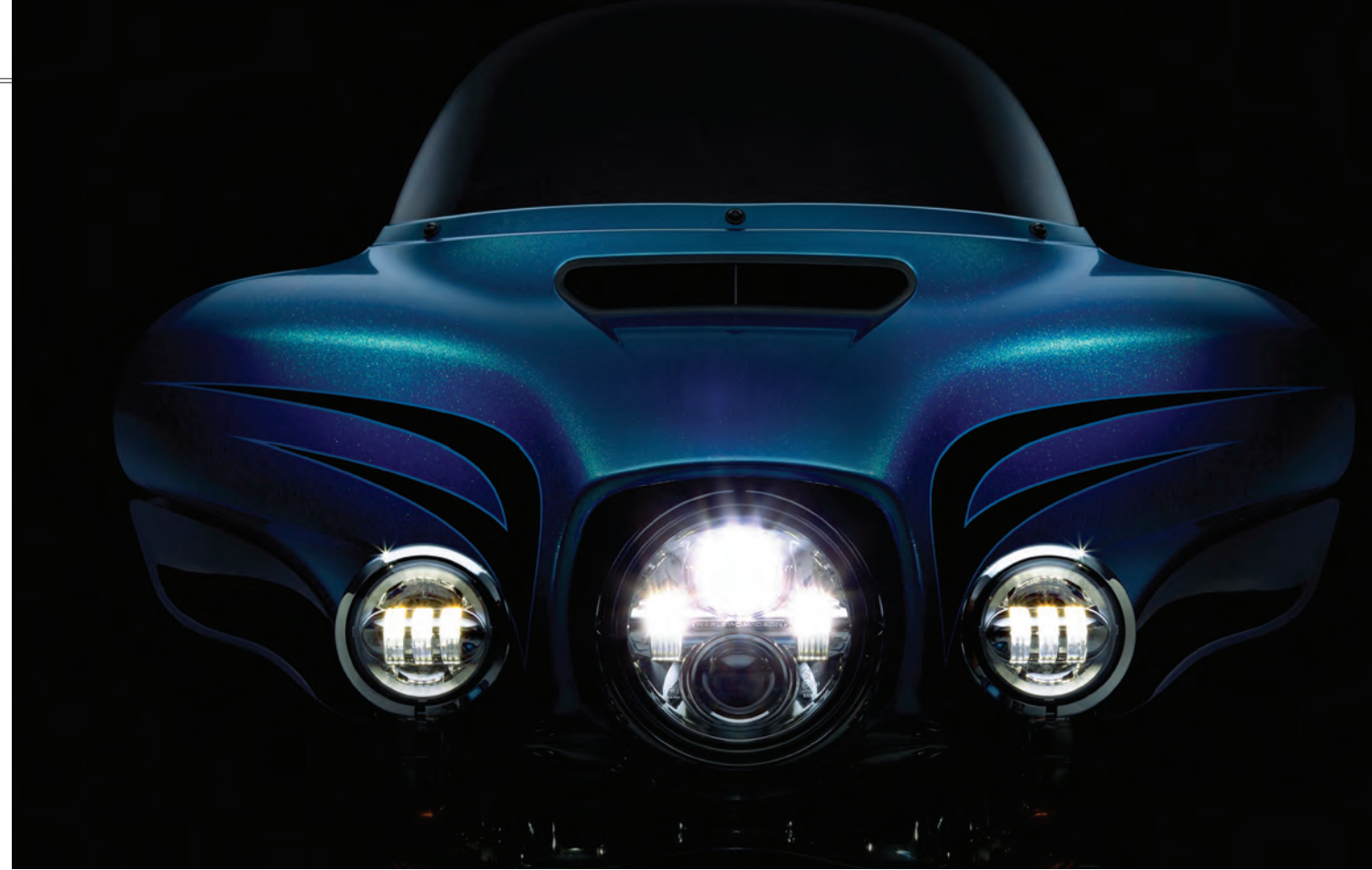
FRONT AND REAR LED LIGHTING increases visibility (above and left); a slimmed-down fender shows off more of the front wheel (below).
