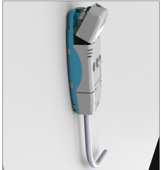
Figure 6. EAFR-01 point sensor mounted to the compartment wall.
