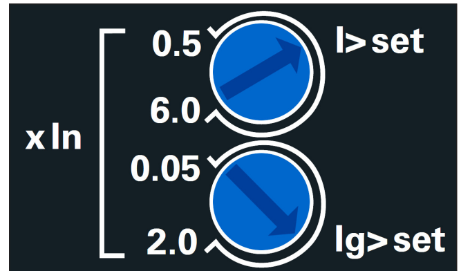
Figure 3. EAFR-110PLV over-current setting potentiometers.
