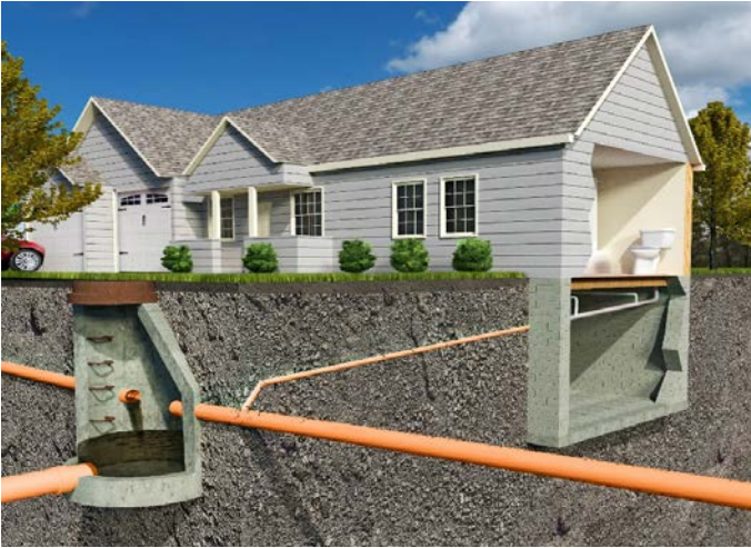
Figure 1 - Lateral To be Lined from Basement Towards Main
