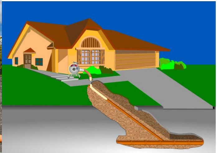
Figure 2 - Lateral Installation from Cleanout
