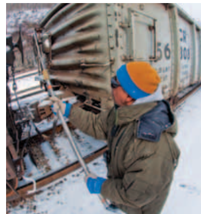
■ Conductor Willie Perry , who works on the Pocahontas Division, uses a telescoping brake stick patented by NS.
