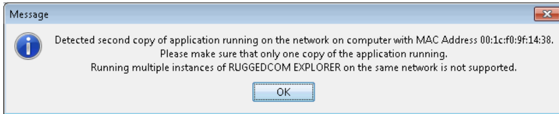
Figure 27: Detecting Another Instance Of EXPLORER On The LAN
