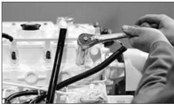
Figure 17: Reinstall injector. Torque to proper tightness.
