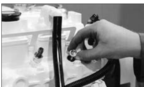
Figure 16: Remove and replace copper sealing washer.
