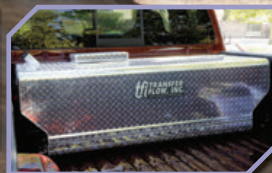
AUXILIARY FUEL TANKS
