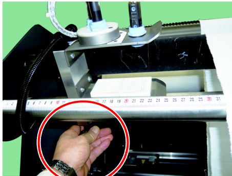
Loosen the finger screw located on the rear surface of the sensor unit to make the sensor unit movable to right and left.
