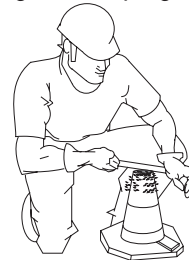
Figure Q. Slump Test (Removing Excess Concrete)
