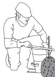
Figure S. Slump Test (Measurement)
