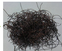
After treatment: Metals left after the organic matter was gasified
