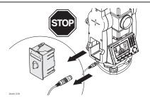
$\ensuremath{\mathsf{Do}}\xspace\, \ensuremath{\mathsf{NOT}}\xspace$  remove the battery during operation of the instrument, or during the shutdown procedure.
