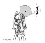
With a horizontal line of sight the vertical circle reading should be exactly 90°(100 gon). The deviation from this value is termed the Vertical index error (i).
