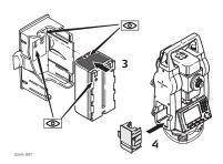
Insert the new battery into the battery holder (3), ensuring that the contacts are facing outward. The battery should click into position.
