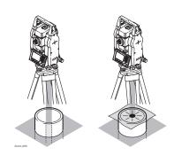
Under some circumstances the laser dot is not visible, for example over pipes. In this case, using a transparent plate enables the laser dot to be seen and then easily aligned to the center of the pipe.
