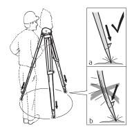
Loosen the clamping screws on the tripod legs, pull out to the required length and tighten the clamps.
