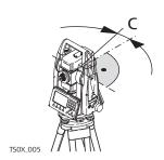
The line-of-sight error (c) is the deviation from the perpendicular between the tilting axis and line of sight. This could be eliminated by measuring in both faces.
