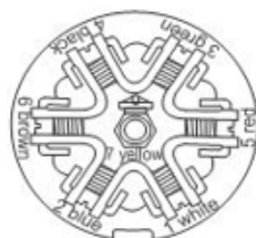
7-way trailer plug car end, rear view
