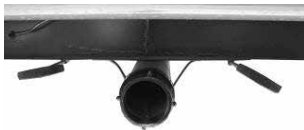
Black/Grey Tank Drain and Valves
