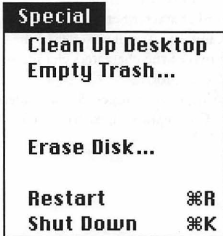
Figure 2-18: The new Special menu now has a keyboard shortcut for Restart (covered later) and Shut Down.
