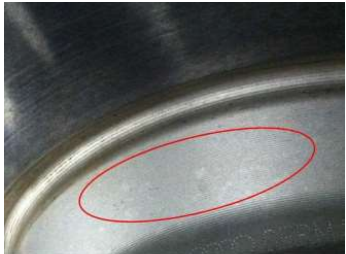
Figure 4. Small spots and discoloration due to chemical contamination from cleaner that was sprayed directly onto the disc.
