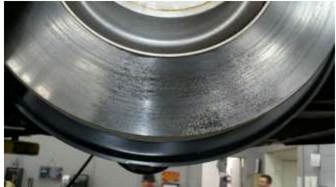
Figure 5. Brake pad material has transferred to the discs.
