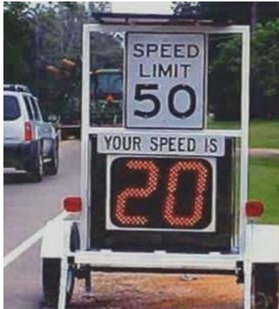
Figure 37. Portable radar speed trailer in San Francisco, California. (Source: Federal Highway Administration ).
