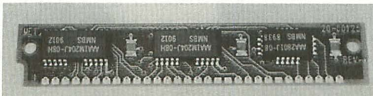
Figure 6-6 Some manufacturers use a combination of PLCC and SOJ DRAM chips.
