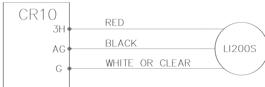
FIGURE 7.1-1. Wiring Diagram for LI200S
